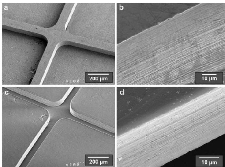
SEM photomicrographs of micro-milled molding master finished with a 100 μm radius milling bit (a, b) and its replicate hot-embossed into PMMA (c, d). The width and depth of the channel, as determined by the dimensions of the mold master, was 100 and 90 μm, respectively
