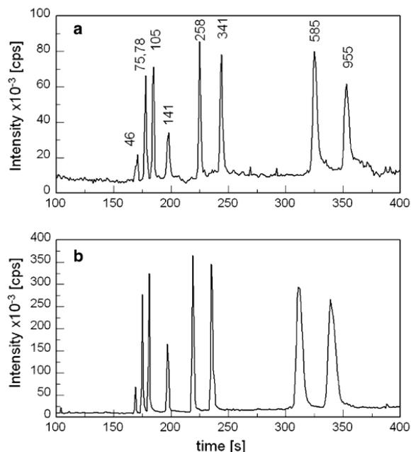
Separation of pUC19 Sau3AI double-stranded DNA stained with 1 μM TO-PRO-3 dye using a PMMA microchip with an offset T injector.  $E_{inj} = 400 \text{ V/cm}$ ;  $t_{inj} = 25 \text{ s}$ ;  $E_{sep} = 110 \text{ V/cm}$ ; separation length 3.5 cm; 4% LPA was used as the sieving matrix. PMMA microchips were hot embossed using either a high precision micro-milled master or b LiGA-made master
